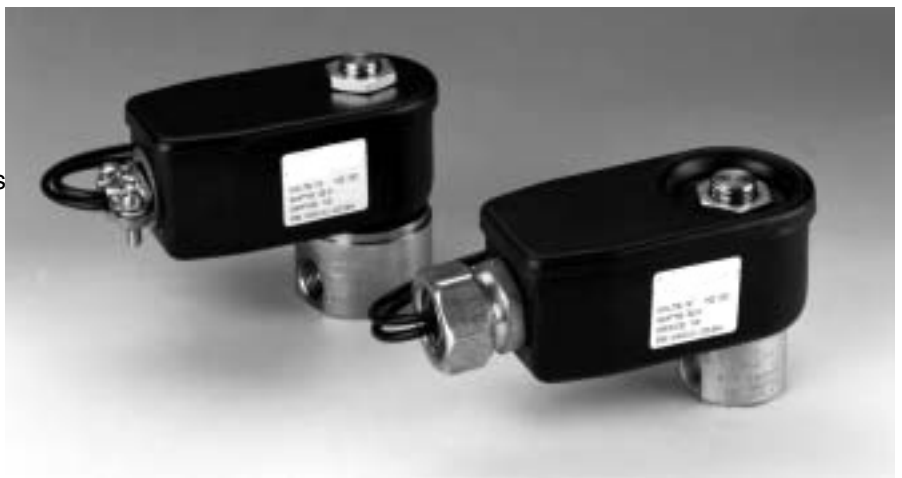
Splice Box option for Coast Series 20 (stainless steel, left) and Series 30 (brass, right) solenoid valves provides space for multiple wiring hookups and an easy access cover for quick and inexpensive field wiring connections directly to the solenoid valve. Splice Boxes shown here with user-provided wire connectors.
